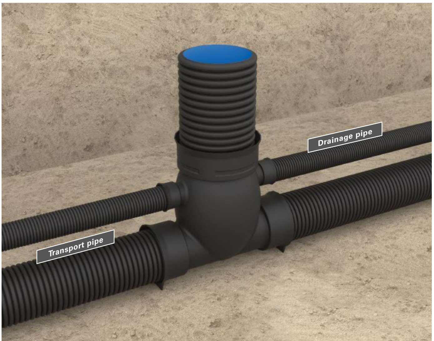
StrabuControl HP with a tight transport pipe at the bottom, and a drainage pipe at the top
